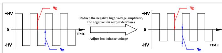
The output frequency of positive and negative ion is adjustable, which is suitable for different discharge distance to achieve faster discharge speed.
