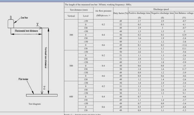
Remarks: 1\*——Real-time pressure value during gas flow. The balance voltage performance of the ion bar varies with the length of the bar, airflow press environmental conditions to make the balance performance of the ion bar reach the best state orking frequency, and installation distance; the duty cycle should be adjusted according to the specific us
