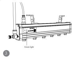
Connect the air source connector on the bar body to the air source generating device, turn on the air source switch and pay attention to the maximum operating pressure of the compressed air flow to avoid malfunction of the ion bar.
