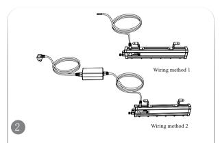
Wiring method 1: Connect through DC24V high-flexible drag chain power cord. Wiring mode 2: Connect one end of the power cord to the DC24V power supply and insert the other end into the NBC power socket on the bar.
