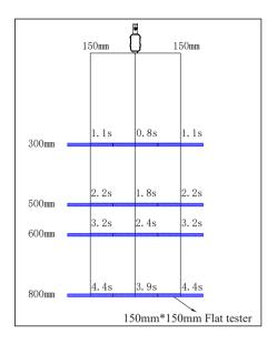
Test Conditions: Ion bar length: 360mm
